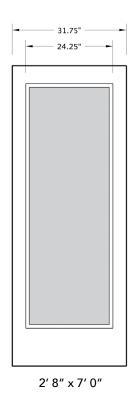
NOTE: BY REQUEST, DOOR HEIGHT COMES IN VARYING DIMENSIONS TO A MINIMUM OF 83". EXCESS WILL BE TAKEN FROM BOTTOM RAIL. ALL OTHER DIMENSIONS WILL REMAIN THE SAME.
